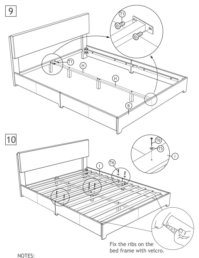
When assembling Part (I), fix the screws on both sides and then the middle.
