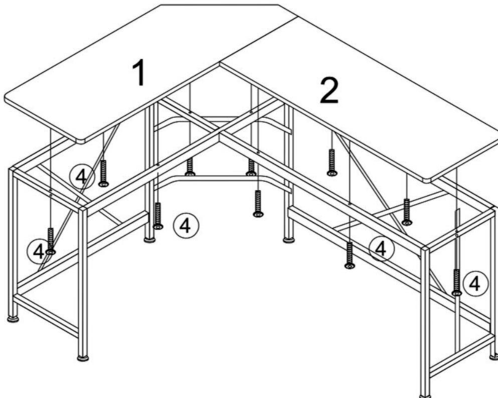
Using the wrong screw can result in a broken desktop.
