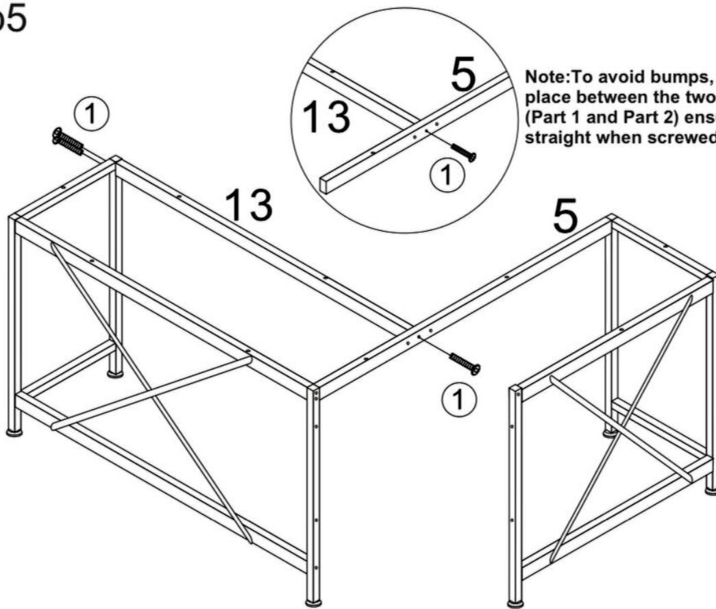
Note: To avoid bumps, place between the two desktops (Part 1 and Part 2) ensure rods 13 and 5 are straight when screwed together.
