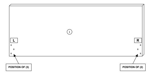
There is a sticker pre-sticked on backside of HEADBOARD SUPPORT RAIL(R)-(2) which marked with R . There is a sticker pre-sticked on backside of HEADBOARD SUPPORT RAIL(L)-(3) which marked with L .
