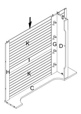
Step 6. Attach left side panel (part B) to assembled unit (part D, F, G, H , J & K) using wood dowels (part #7) then lock the hardwares.
