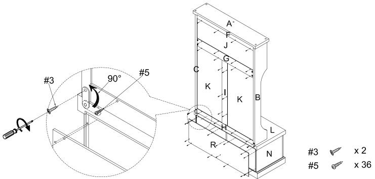
Step 15. Attach hinges (part #11) to door (part Q), lower left side panel (part N) and lower right side panel (part O) using flat head screws (part #3) and Phillips head screwdriver.
