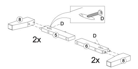
Use screw (D) to attach part (5) to part (8) and attach part (6) to part (8), do this step twice
