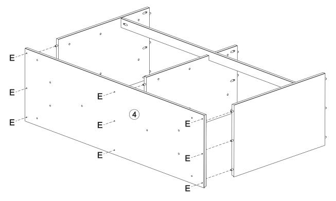
Attach part (4) to body with screws (E)
