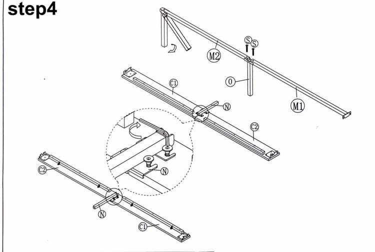
Put the part "N"on part "C1"and part "C2".
