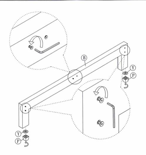
Loosen the pre locked screws.
