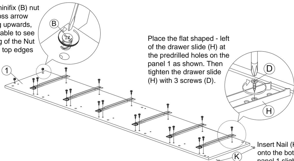
Place the flat shaped - left of the drawer slide (H) at the predrilled holes on the panel 1 as shown. Then tighten the drawer slide (H) with 3 screws (D).
