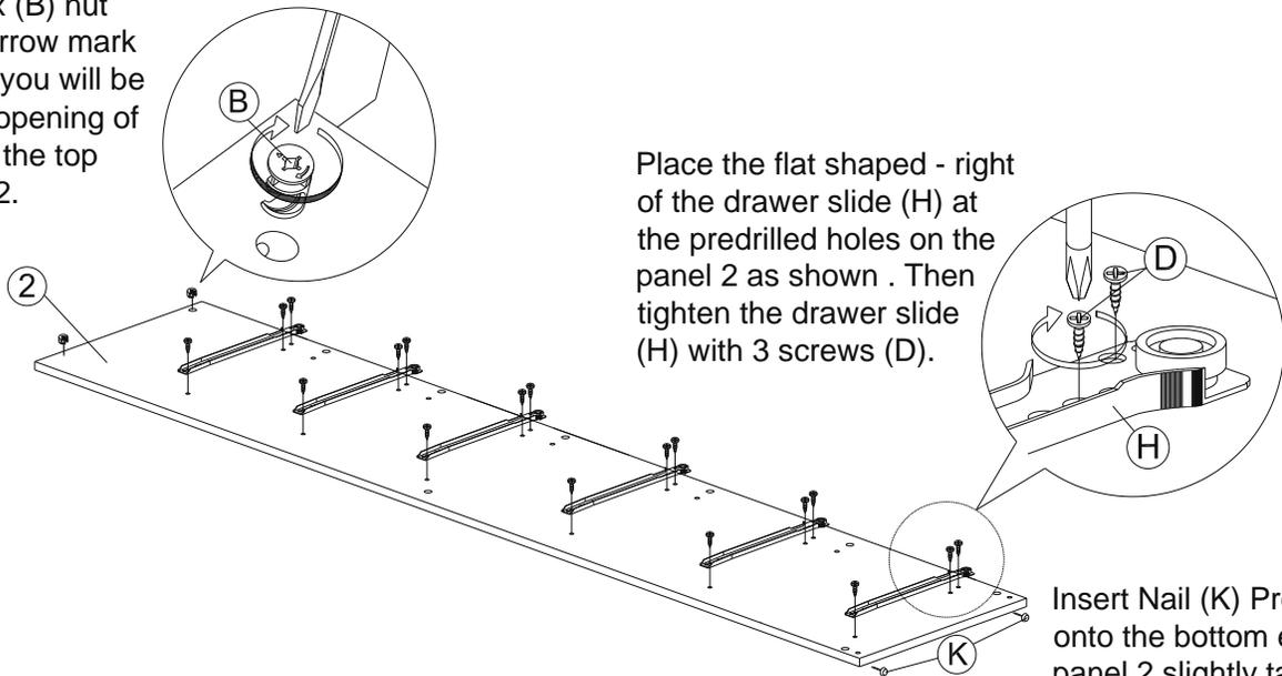
Place the flat shaped - right of the drawer slide (H) at the predrilled holes on the panel 2 as shown . Then tighten the drawer slide (H) with 3 screws (D).
