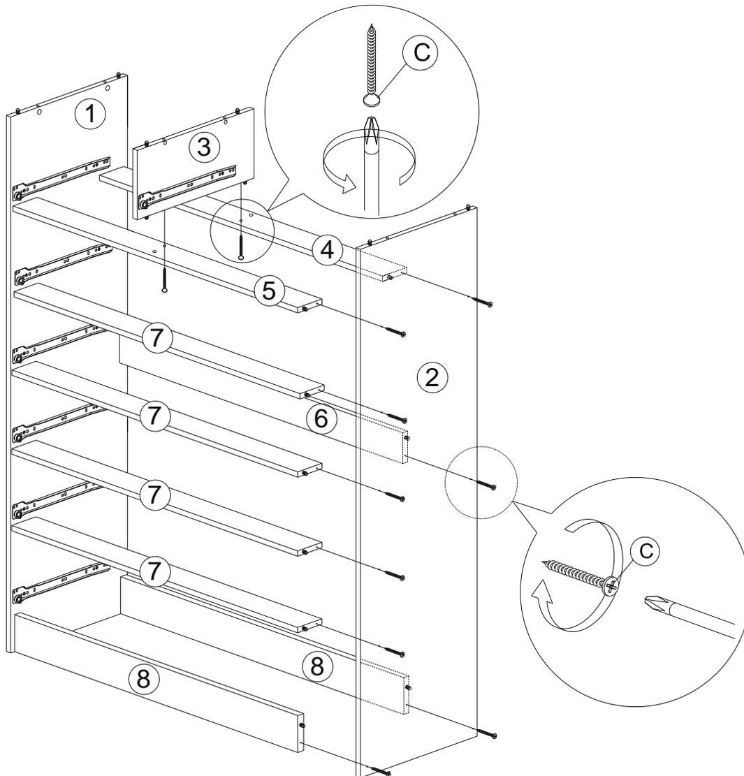
\*Place and fix panel 4,5,6,7 and 8 onto panel 2 by inserting the (Right) dowels onto the non-thru holes at panel 2, then slightly hammer it in from outside of panel 2.
