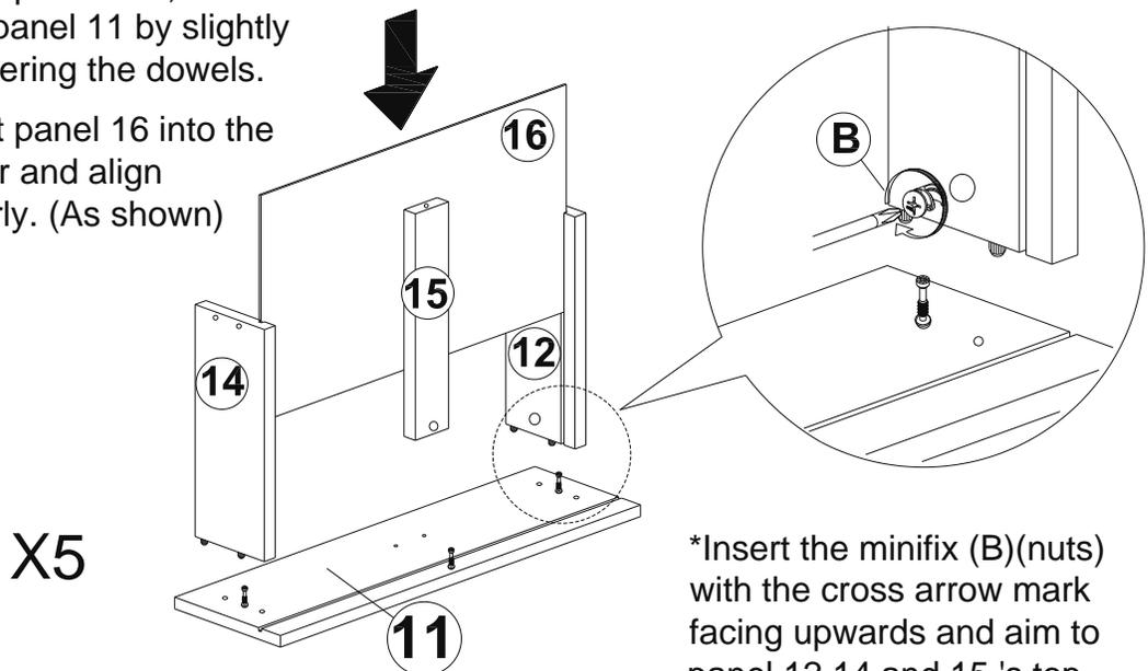
\*Insert the minifix (B)(nuts) with the cross arrow mark facing upwards and aim to panel 12,14 and 15 's top thru holes.(As shown)
