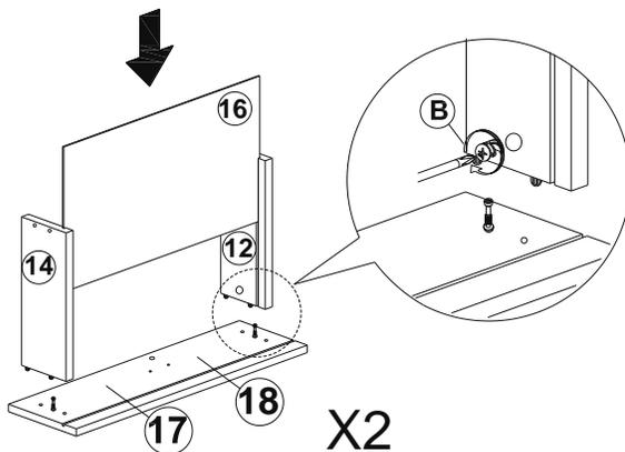
\*Insert the minifix (B)(nuts) with the cross arrow mark facing upwards and aim to panel 12 and 14 's top thru holes.(As shown)
