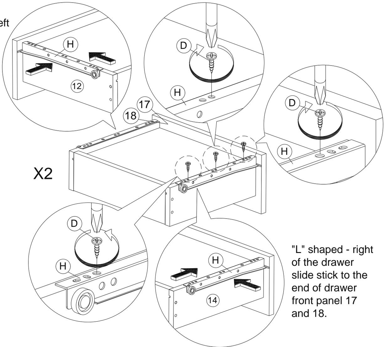
"L" shaped - right of the drawer slide stick to the end of drawer front panel 17 and 18.
