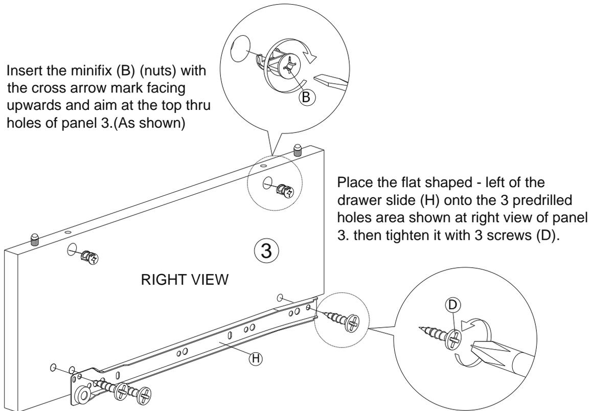
Place the flat shaped - left of the drawer slide (H) onto the 3 predrilled holes area shown at right view of panel 3. then tighten it with 3 screws (D).
