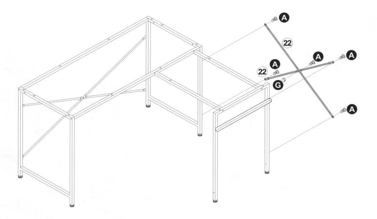
Note: Keep guide rails on Metal Frames 11 and 10 in the corresponding direction.
