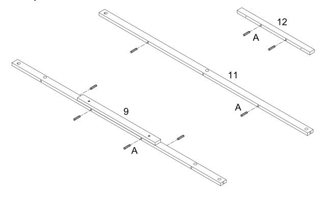
Insert the wooden dowel (A) into the front panel (9,11,12).
