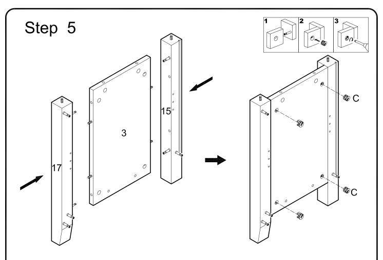
Use cam lock (C) to assemble the wooden legs (15,17) to the side panel (3).
