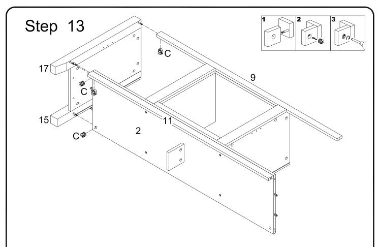
Assemble the wooden leg (15,17) to the front & bottom panel (2,9,11) and secure it with cam lock (C).
