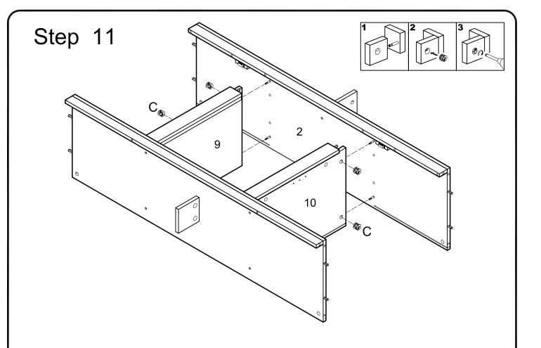
Use cam bolts (C) to secure the middle panel (2) into the support panel (9,10).
