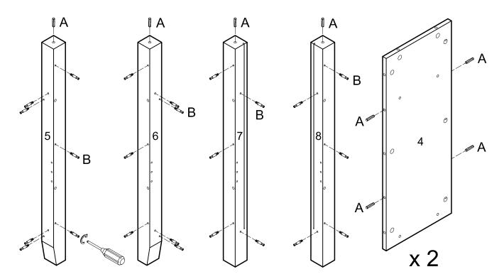
Insert the wooden dowel (A), and cam bolt (B) into the wooden legs (5,6,7,8). Insert the wooden dowel (A) into the side panel (4).
