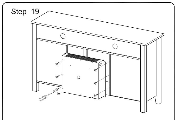
Attach the fireplace insert (D) to the stand by securing it with screw (E).
