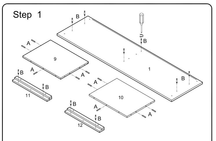
Insert the wooden dowel (A) into the support panel (9)(10). Insert the cam bolt (B) into the top panel (1), face plate (11)(12).
