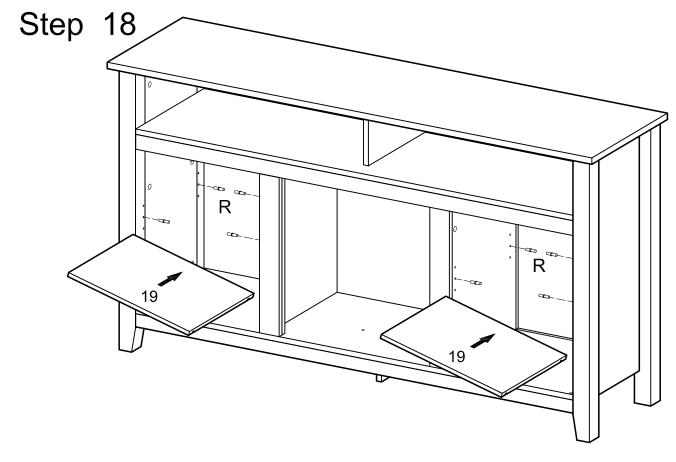
Insert the shelf support pin (R) into the stand and place the wooden shelf (19) on top.
