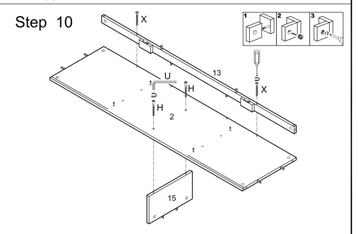
Turn the middle panel (2) upside down and use cam lock (C) to secure the skirt (13). Use screws (H) and wrench (U) to attach the support panel (15).
