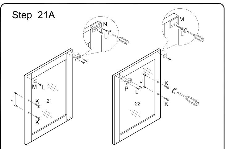
Attach the door hinge (N) and metal plate (M) to the glass doors and secure it with screw (L). Attach the door Handle (J) to the doors and secure it with handle bolt (K).
