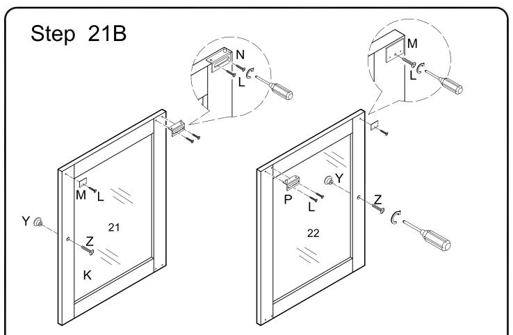
Attach the door hinge (N) and metal plate (M) to the glass doors and secure it with screw (L). Attach the door knob (Y) to the doors and secure it with knob bolt (Z).
