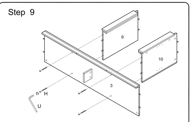
Attach the side panel (9,10) to the bottom panel (3) and secure it by bolt (H) and wrench (U).
