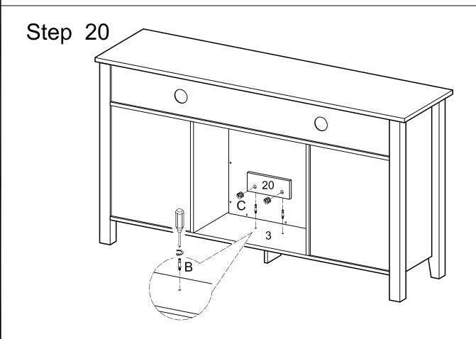
For security, insert the cam bolts (B) into the bottom panel and use cam lock (C) to attach the support panel (20) to the bottom panel (3).
