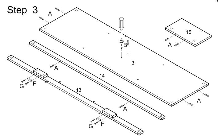
Insert the cam bolt (B) and wooden dowel (A) into the bottom panel (3.). Insert the wooden dowel (A) into the skirt (14) and support panel (15). Attach the door stopper (F) to the skirt (13) and secure it by screw (G).
