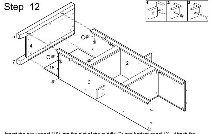
Insert the back panel (18) into the slot of the middle (2) and bottom panel (3). Attach the wooden leg (5,7) to the middle panel (2), bottom panel (3) and skirt (13)(14) and secure it with cam lock (C).
