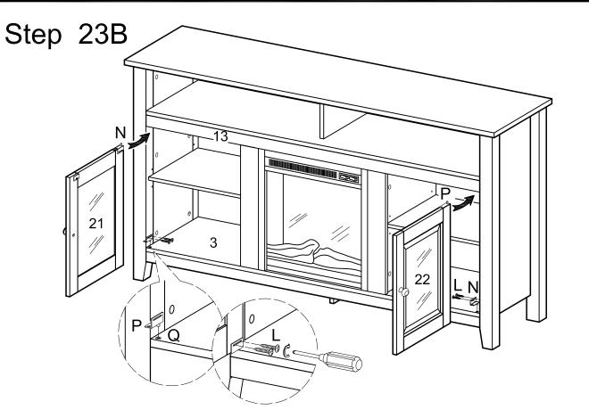
Insert the door hinge (P) into the plastic pivot (Q) on the bottom panel (3). Attach the door hinge (N) to the plastic pivot on skirt (13) and secure the door hinge (P) with screw (L).
