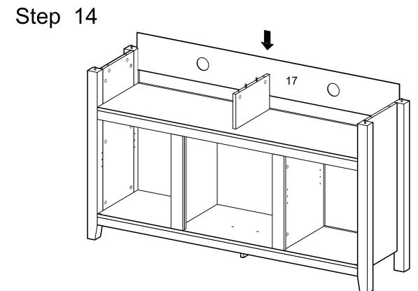
Place the stand up right and place the back panel (17) in the slot in the legs.
