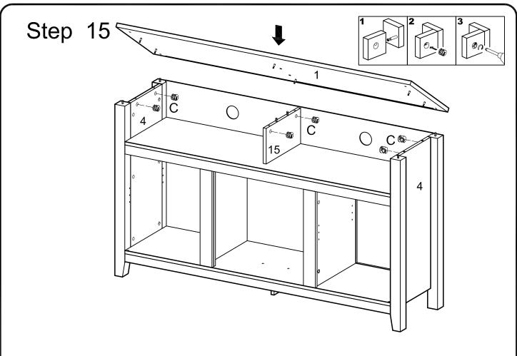
Place the top panel (1) on the stand and secure it with the cam locks (C).
