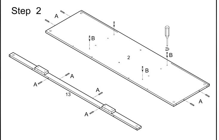
Insert the wooden dowel (A) and cam bolt (B) into the middle panel (2). Insert the wooden dowel (A) into the skirt (13).
