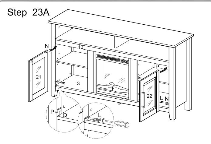
Insert the door hinge (P) into the plastic pivot (Q) on the bottom panel (3). Attach the door hinge (N) to the plastic pivot on skirt (13) and secure the door hinge (P) with screw (L).
