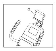
**holder.** If applicable to your tablet holder model, rotate and/or pivot the tablet holder to the desired position. Reverse these actions to remove the tablet from the tablet holder.
