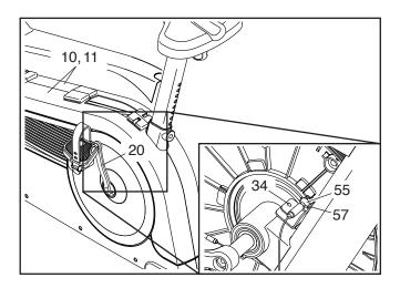
Then, carefully pull the tops of the Shields (10, 11) apart and locate the Reed Switch (57). Rotate the Left Crank Arm (20) until a Magnet (55) is aligned with the Reed Switch. Then, slightly loosen the #8 x 18mm Screw (34), slide the Reed Switch slightly toward or away from the Magnet, and then retighten the #8 x 18mm Screw.
