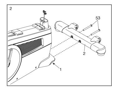
3. Attach the Rear Stabilizer (3) to the Frame (1) with two M10 x 110mm Screws (53).
