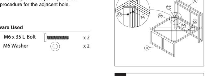
2. Align all four holes of the side frame (C). For each hole, insert M6 x 35 L bolt (AA) through M6 washer (CC), the seat frame (B) and back frame (A). Repeat this step for the oposite side. Do not tighten completely. Repeat this procedure for the adjacent hole.
