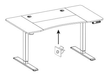
Install K -AC Adapter,B -Controller and L -Wire Basket on the desktop.
