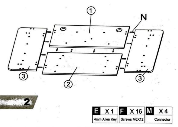
Note: The horizontal bar on the connector should be perpendicular to the seam of table panel slice
