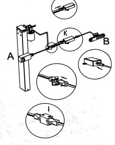
Stand the desk up, press the outlet box firmly into the desktop and use the wire clips to tide up wires
