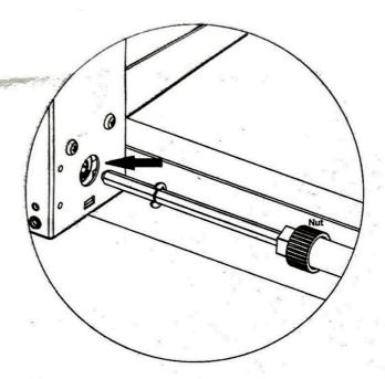
Secondly, put the other side of the coupling rod into the pre-built rod on the motor leg and then lock the plastic nut again.
