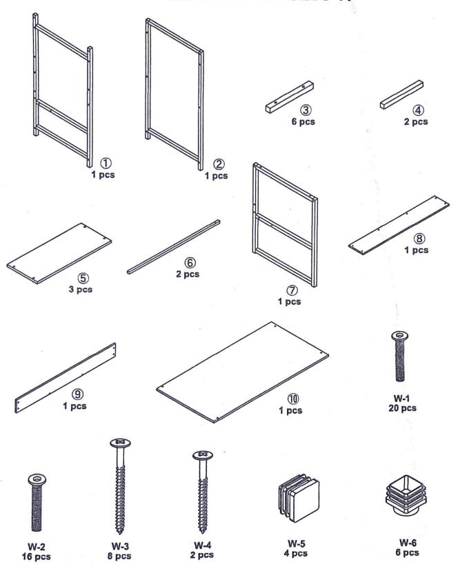
Notes: Don't tighten screws completely at first, just in case parts were assembled wrong and need disassembled. Tighten screws at last when all parts are put together.
